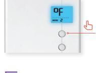
Press and release UP or DOWN button to select the desired setting value
