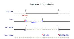
The figure above shows how the timing works at a long activation, where the activation must be longer than the time specified in configuration parameter 17 to be accepted as a long activation (Central Scene Key Held).
