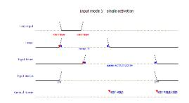
As illustrated above, a KEY HELD Central Scene notification will appear even though the activation on the input is shorter than configuration parameter 17. This is because the status on the input is prolonged with the time specified in the configuration parameter for the input timer (parameter 4/6/8/10/12/14).
