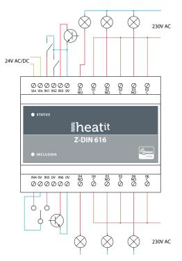
The Heatit Z-DIN 616 must be connected to a 24 Volt AC or DC power supply via the terminals labeled "Vin". The polarity is of no importance. The supply must be dimensioned to allow the supplied module with enough power to enable all relays to be activated. Regarding power consumption: see the technical details section.
