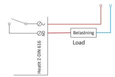
The 6 outputs of the Heatit Z-DIN 616 module consist of 1-pole SPST connectors (Single-Pole Single-Throw).
