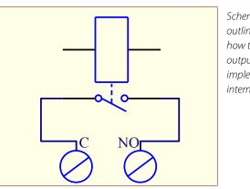
Schematic outlines of how the relay outputs are implemented internally
