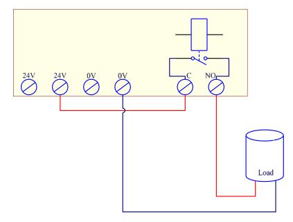
Schematic outline example of how the 24V supply output, together with a relay output, can be used to control a load.
