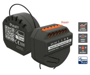
Heatit ZM Thermostat is an electronic thermostat for electrical underfloor heating designed for inwall installations. The thermostat allows you to control your electrical heating through your Z-Wave network. The module is equipped with a 16A single pole relay. The thermostat requires you to connect an external wired sensor which is included with the device. The device can withstand a max load of 16A at 230VAC.
